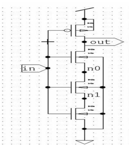
**Figure (5)** Forced 2-NMOS CMOS inverter
