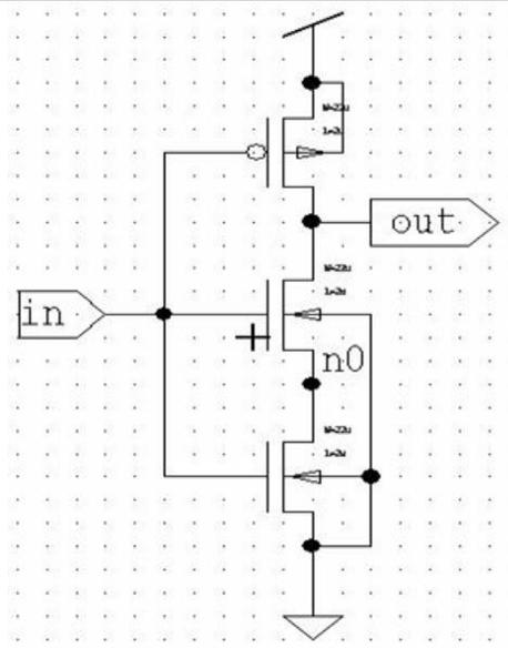
**Figure 3:** Forced NMOS transistor inverter
