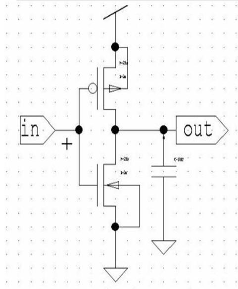
**Figure 2:** Conventional CMOS inverter CMOS
