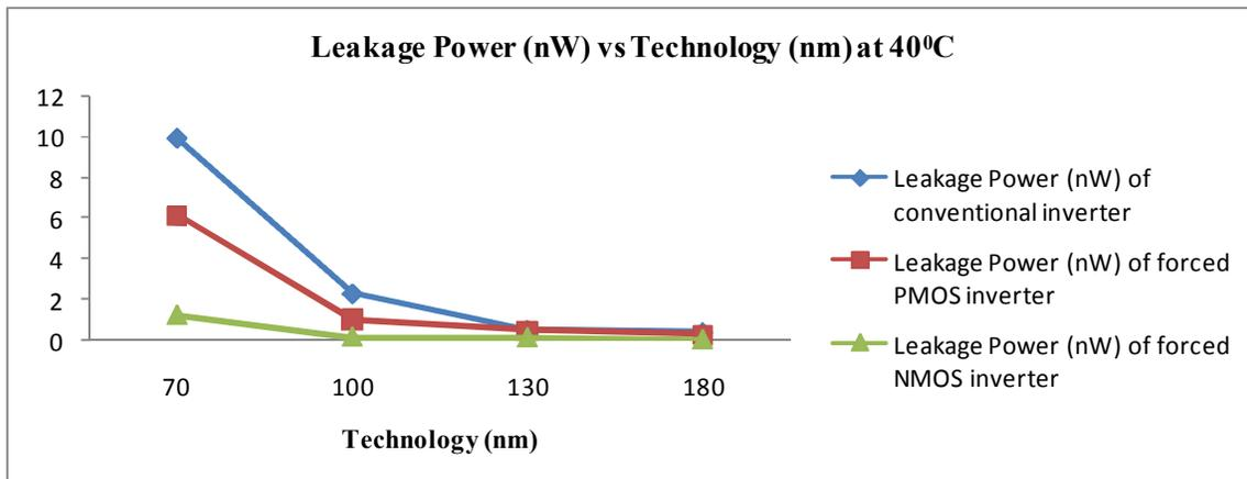
Figure 8: Leakage Power vs. Technology curve
