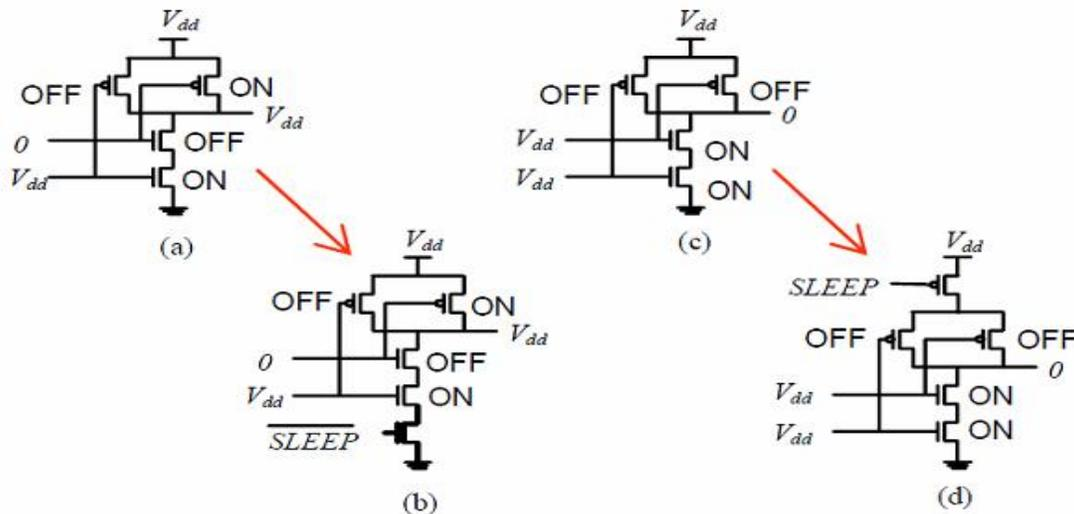
Figure 2 Reducing the leakage using stacking
