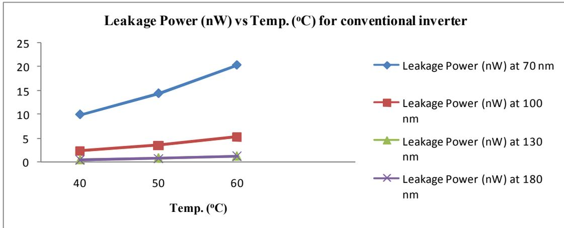
Figure 6: Leakage Power vs. Temperature at different technologies curve
