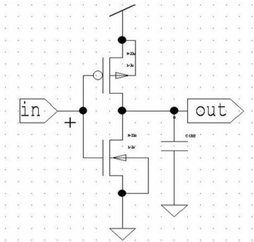
Figure 3: CMOS Inverter
