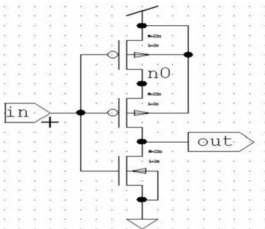
Figure 5: CMOS forced PMOS Inverter
