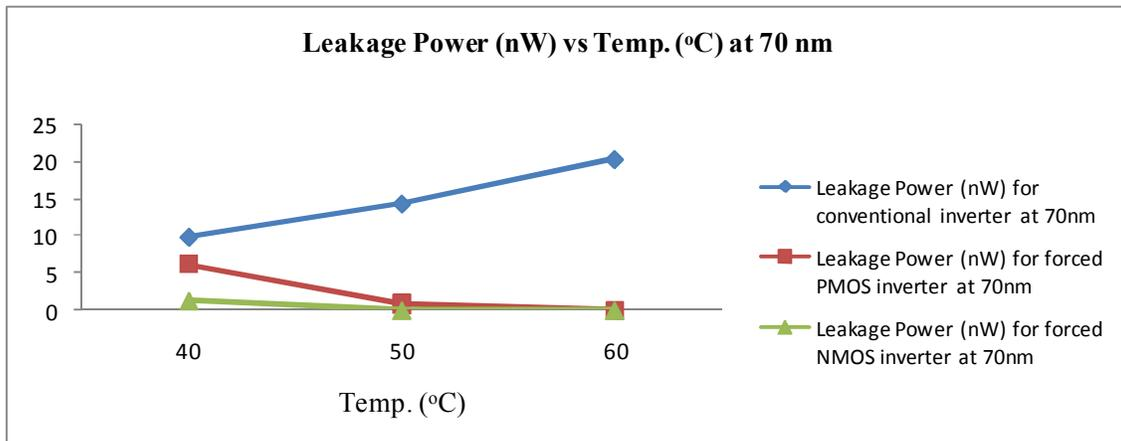
Figure 7: Leakage Power vs. Temperature at 70nm curve
