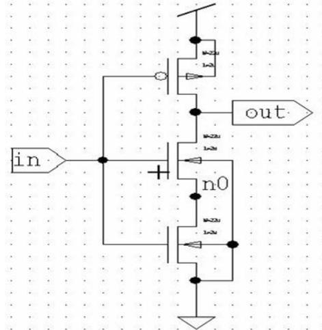
Figure 4: CMOS forced NMOS Inverter
