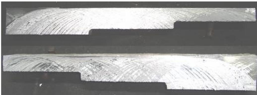
**Figure10:** Section of casting shows no shrinkage defect
