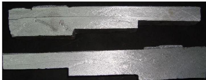
**Figure16:** Section of casting shows no shrinkage defect.
