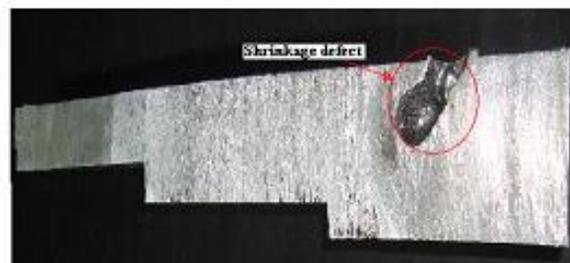
**Figure7:**Section of casting with shrinkage defect
