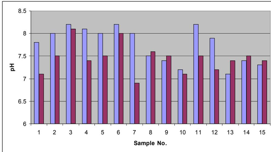
**Figure 2:** Graphical presentation of pH in shallow and deep aquifers
