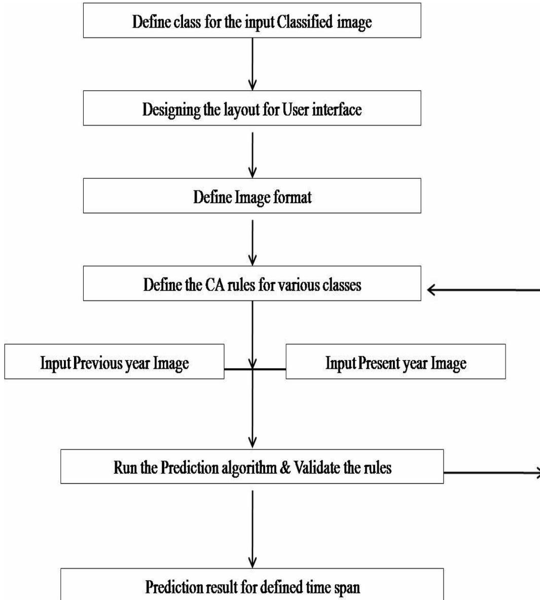
**Figure 2:** Flowchart for Cellular Automata algorithm
